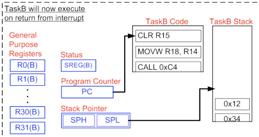
The RTOS tick interrupt interrupted TaskA, but is returning to TaskB - the context switch is complete!
