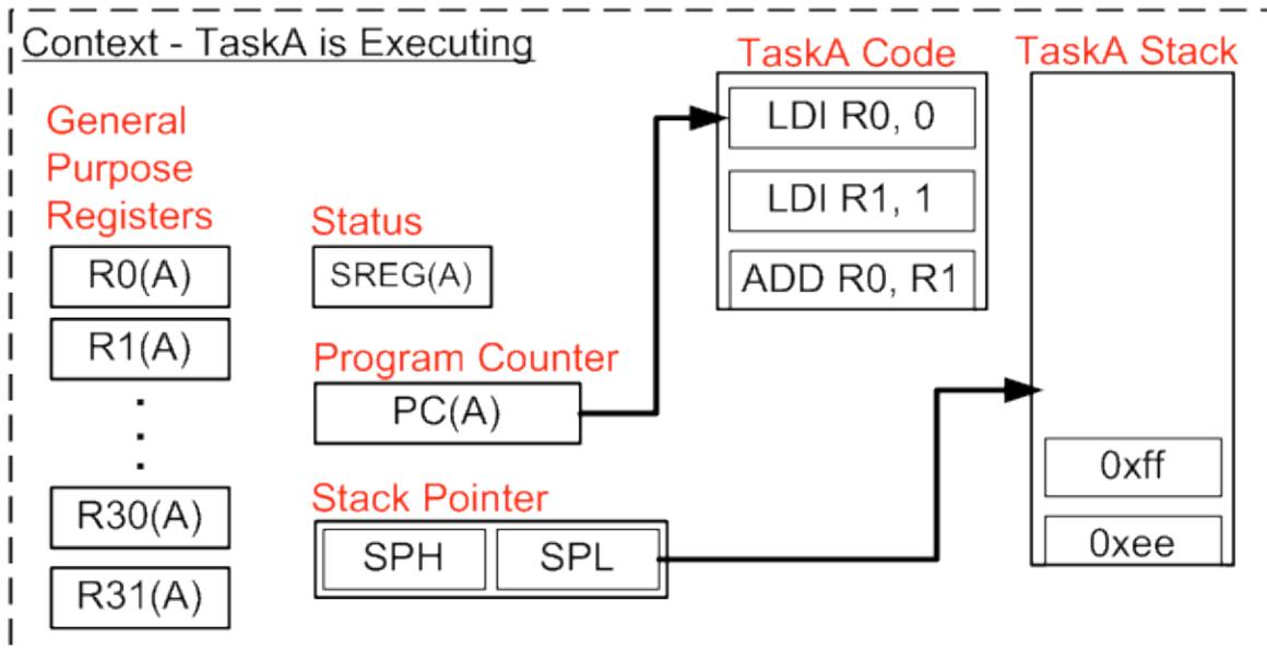
The (A) label within each register shows that the register contains the correct value for the context of task A.
