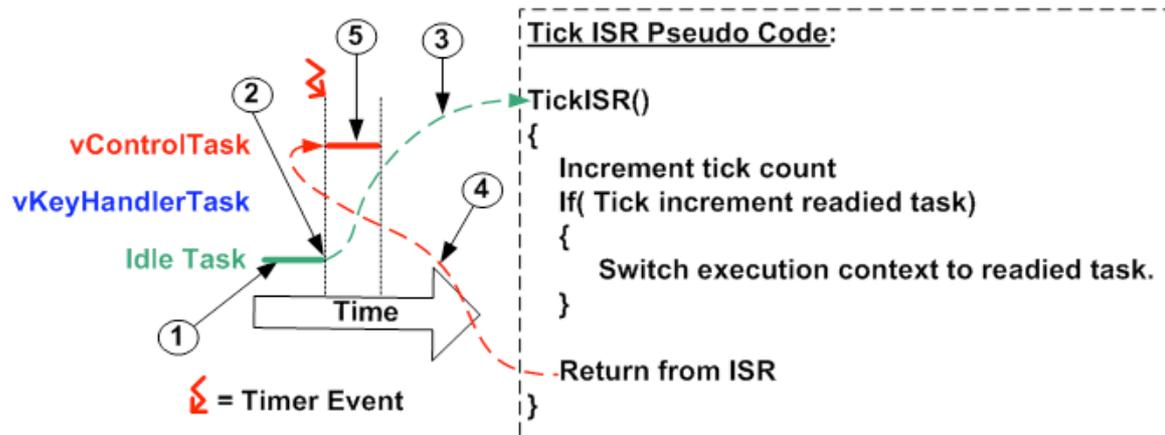
In this type of diagram time moves from left to right. The coloured lines show which task is executing at any particular time. Referring to the numbers in the diagram above:
